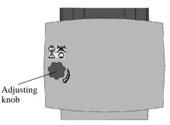
Turn adjusting knob in a clockwise direction with the motor running until scraping noises are heard and fine aluminium chips fall out of the delivery chute. Worn points on the shaving plate are optimally compensated.
